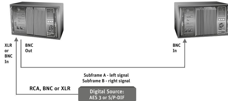
**Connecting multiple KH 310 D loudspeakers together**
